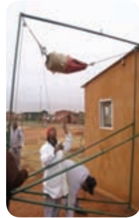
SABS soft body impact testing
