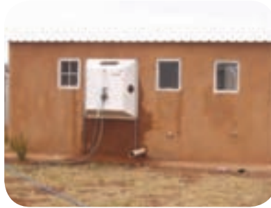
SABS rainwater penetration testing
