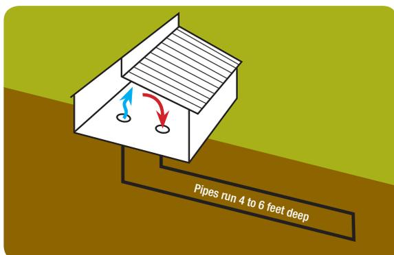
This figure presents an open-loop air-tube system used for both cooling and heating.
